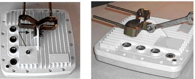
3. Raise mounting bracket to proper angle and tighten carriage bolt. Use a nut driver or socket wrench to firmly tighten the carriage bolt.
